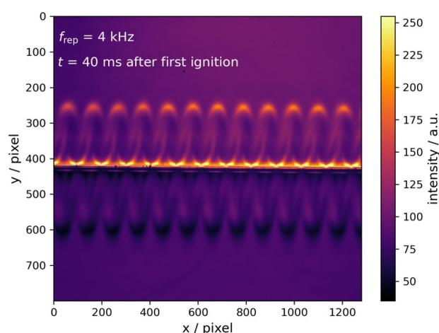
**Figure 1:** Exemplary lateral schlieren image of a SDBD source during the transient start phase.
