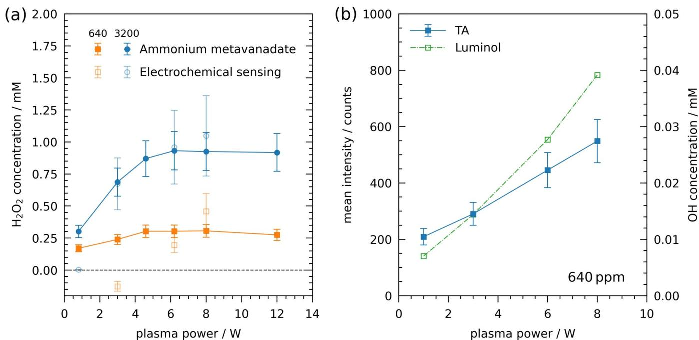
**Figure 1:** (a) H<sub>2</sub>O<sub>2</sub> concentration as a function of plasma power at humidity concentrations of 640 ppm and 3200 ppm, measured with a spectrophotometric approach using ammonium metavanadate and electrochemical sensors. (b) OH distribution measured by chemiluminescence of luminol and OH concentration measured by terephthalic acid (TA) dosimeter as a function of plasma power at a humidity of 640 ppm.
