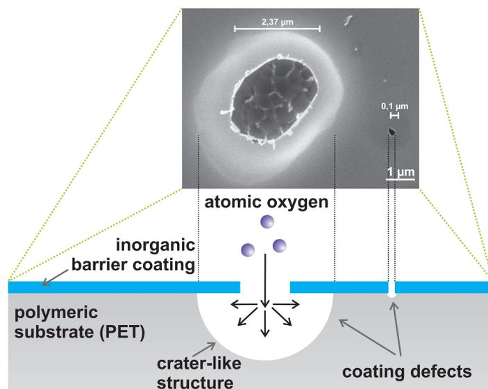
Figure 3: Schematic illustration of coating defect visualization by oxygen etching in a reactive plasma.
