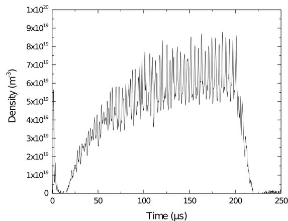
Figure 2: Evolution of the measured electron density during a single HiPIMS pulse. The oscillations are caused by the spokes moving over the probe.
