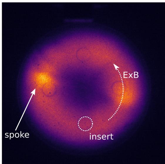
Figure 1: False color image of the discharge in front of the target. The 4 probes inside the target surface can be seen as dark outlines. Two spokes rotate in the marked direction.
